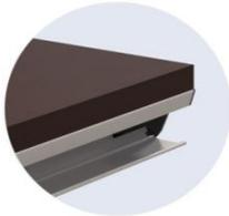
Tap-in Powerway is constructed from 16 gauge sheet metal that has been formed into a U-shaped trough, punched with wire access ports and clearance holes to accommodate mounting hardware. The Tap-in Powerway door is formed 16 gauge sheet metal that is attached on to the U-shaped trough with hinged springs.
