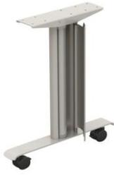
1/16" Extruded aluminum forms the door and the outer shell of the Vertical Wire Manager. The door is connected to the outer shell with a ball and socket hinged joint. The Vertical Wire Manager attaches to the table leg column with two zinc die cast U-clips that are mechanically fastened to the outer shell. The door closes with a friction fit.
