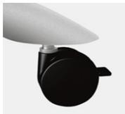
Casters are twin wheel and made of a durable nylon pneumatically attached to a 5/16"- 18 threaded steel insert which is threaded into solid 1/2" diameter steel nutsert machined to accept 5/16" -18" threads.
