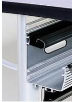
Extruded .100" wall aluminum J-shaped trough, punched with wire access ports and clearance holes to accommodate mounting hardware is the basis of the wire management trough. Integrally extruded grooves accept polymer extrusion for additional wire management within the trough. Both the J-shaped trough and the steel door may be finished in any of the Spectone finishes.
