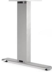
1/16" Extruded aluminum forms the door and the outer shell of the Vertical Wire Manager. The doorsnaps on to the outer shell. The Vertical Wire Manager attaches to the table leg column with two zinc die cast U-clips that are mechanically fastened to the outer shell. The door closes with a friction fit.
